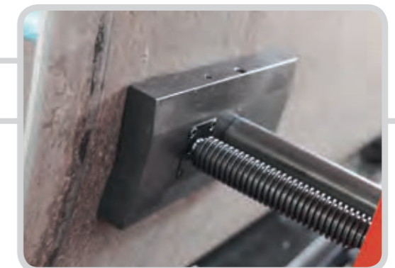
Locking system with 8 independent wide pads.
