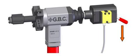
After having supplied the pneumatic locking device with air, move the lever downward to move the locking piston forward that must be 2mm inside from the end of the reduced guiding shaft as show in the picture here below.
