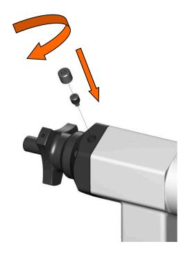
Screw back in the grub screw and the grub screw cover locking them tight.
