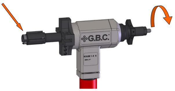
While holding the three LOCKING JAWS you have just mounted, unscrew the VANE EXPANSION NUT in order to let them enter their seat. If the procedure is correctly made the locking jaws should have a little play.
