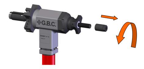
Unscrew the vane expansion nut.
