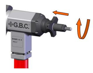
Screw back on the vane expansion nut all the way.
