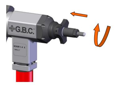
Screw back on the vane expansion nut all the way.
