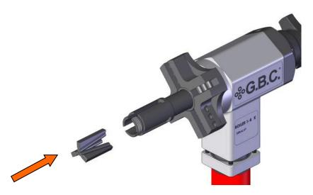
Select the **LOCKING JAWS** according to the diameter of the pipe and install them on the expansion shaft as shown in the picture.
