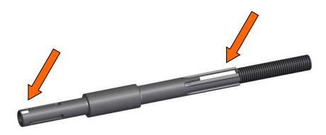
Take the guiding shaft from the reduced shaft kit and mark the groove of the lap joint as well as the far end of the shaft as shown in the picture.
