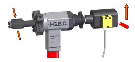
After having supplied the pneumatic locking device with air, keep the locking jaws pressed with your hand and move the lever upward to get the expansion shaft withdrawn in the machine.
