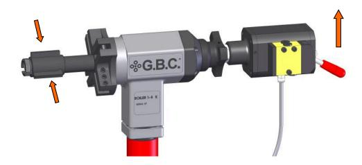
After having supplied the pneumatic locking device with air, keep the locking jaws pressed with your hand and move the lever upward to get the expansion shaft with drawn in the machine.
