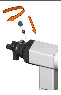
Reassemble the grub screw and the grub screw cover locking them tight.
