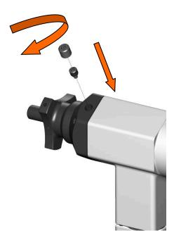
Reassemble the grub screw and the grub screw cover locking them tight.
