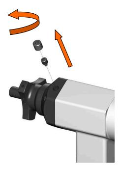
Remove the grub screw cap and the grub screw from the cover case in order to release the guiding shaft.
