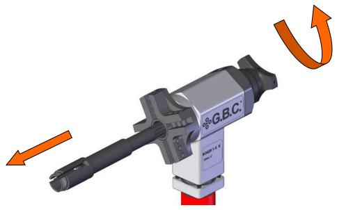
Remove the shaft by rotating the hand wheel clockwise.
