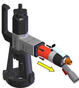
Remove the 4 screws located on each corner of the square flange as shown above.
