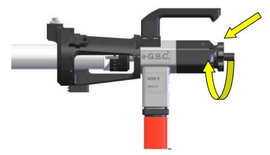
Turn the feeding hand wheel clockwise to move the chuck towards the pipe and as soon as the tools begin to work, reduce the feeding rate to a comfortable feeling, trying to maintain a constant feeding ratio.
