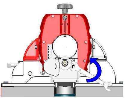
Unscrew the locking nut with a counter-clockwise movement using the wrench supplied with the machine.
