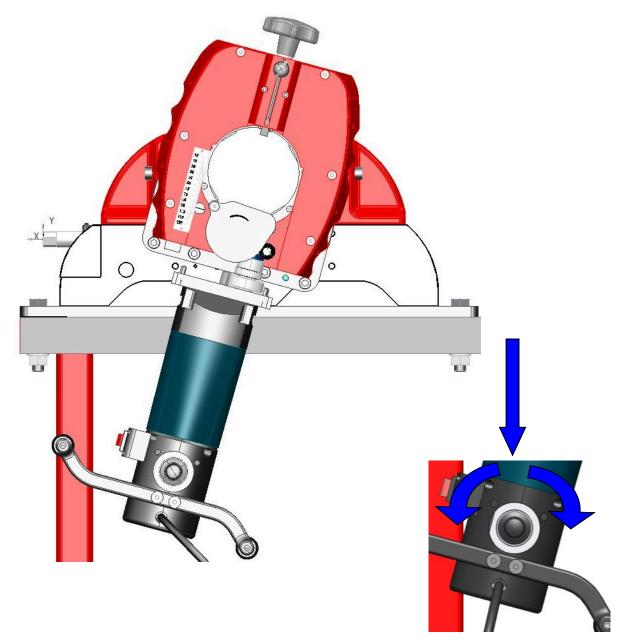
The milling tool speed can be adjusted in function of the type of material and the thickness of the pipe, by rotating the speed regulator knob located on the lower part of the motor.
