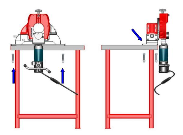
After the machine has been removed from its packaging, position it on top of a working bench as shown in the picture. Once found a satisfactory position fix it in place with N° 4 M16 nuts with suitable length (not included).
