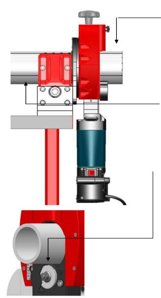
The machine shown in the drawing is intended to be used for cutting pipes with small diameters which are workable with this unit.
