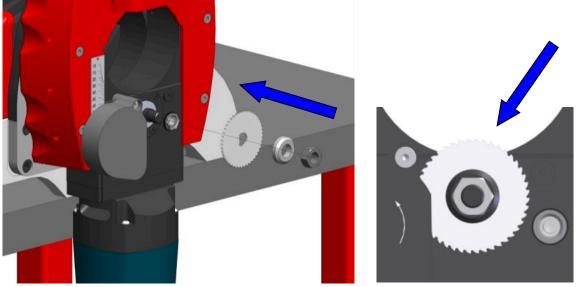
Install the milling tool suitable for the job making sure it is well greased for a better grip, paying attention to the direction of the cutting teeth which must be exactly as shown in the picture.
