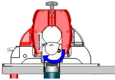
Rotate the protection as shown in the picture.
