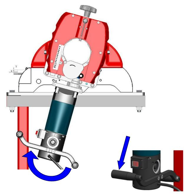
Begin the cutting operation by slowly rotating the machine clockwise on its axis. See the operation shown in the picture.
