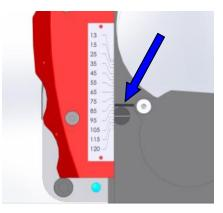
By rotating the hand wheel, position the machine in correspondence of the desired diameter of the pipe to be worked, in a scale value included between 13 and 120mm. The vernier applied on the side of the machine will grant you the maximum accuracy.
