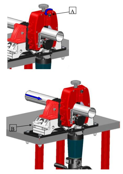
Unscrew the locking screw "A" with a counter-clockwise rotation and pull the reference needle down on the pipe to visually check where the cut will be executed. Now you can lock the pipe in the jaws by acting on the locking nut with the elbow pipe wrench. Now you can set back in place the reference needle and fasten the locking screw to hold it in place.
