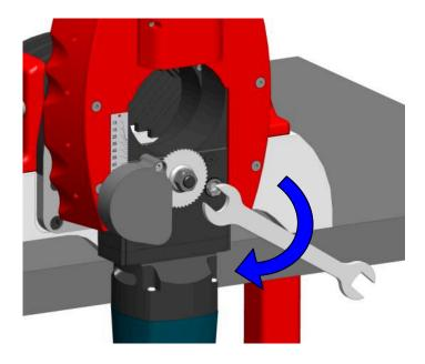
Once the milling tool is installed fasten the bolt with the wrench rotating clockwise.
