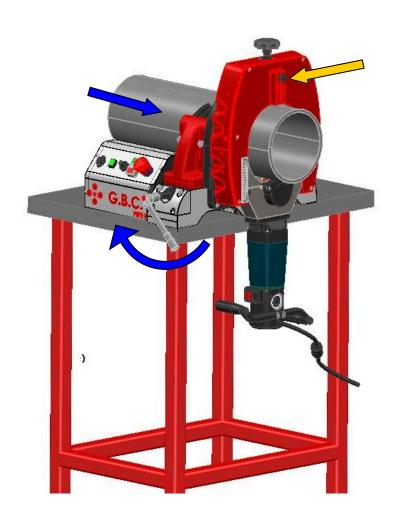
Turn counter-clockwise the knob located on the upper front part of the machine to release the cut point indicator. Now push the pipe into the machine until the cut point desired gets perpendicular to the cut point indicator. Lock the pipe by turning the screw on the side .
