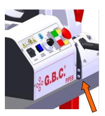
Take the rotation motorized kit out of the package and place it on the workbench as shown in the above picture. Insert the motorized kit in the shaft seat, and once the position is definitely chosen, fix it in place with the 4 screws supplied with the lit itself.
