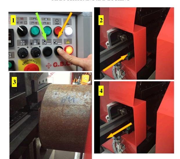
1 -2) Press the pipe positioner "**DOWN**" button to move the pipe positioner between the pipe and the chuck.
