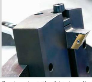
The unit is equipped with easily interchangeable tools for any angle of bevel which come in various hardness scales in relation to the material typology:
