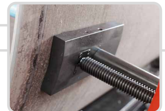
Locking system with 8 independent wide pads.
